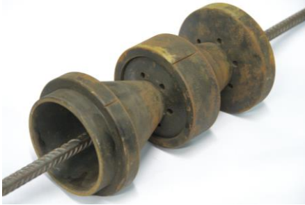
Figure 4 Nozzle assembly used for spraying water onto the bar surface (Courtesy: ARS Steels and Alloy International Pvt. Ltd., Chennai, India)
